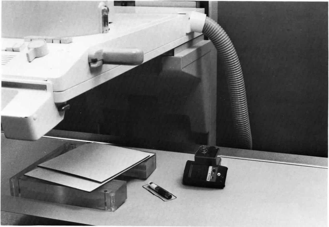
Figure 9.6. Maximum fluoroscopic exposure rate test setup for undertable tubes with a pen dosimeter. Although pen dosimeters are not recommended, it is possible to use them. It is necessary to locate the center of the field and mark this with paper clips so the dosimeter can be replaced in the exact center without fluoroscopic exposure.
