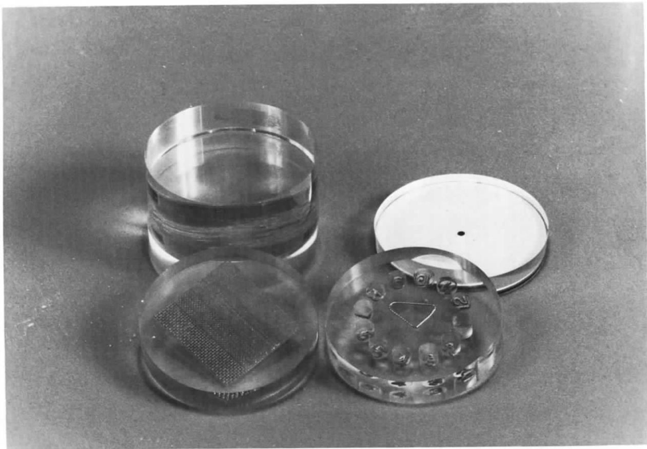
Figure 10.4. Commercially available tomographic phantom. This phantom requires several exposures to obtain the necessary information.
